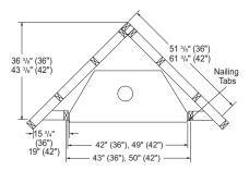
Figure 5 - Framing Clearances for Corner Installation
